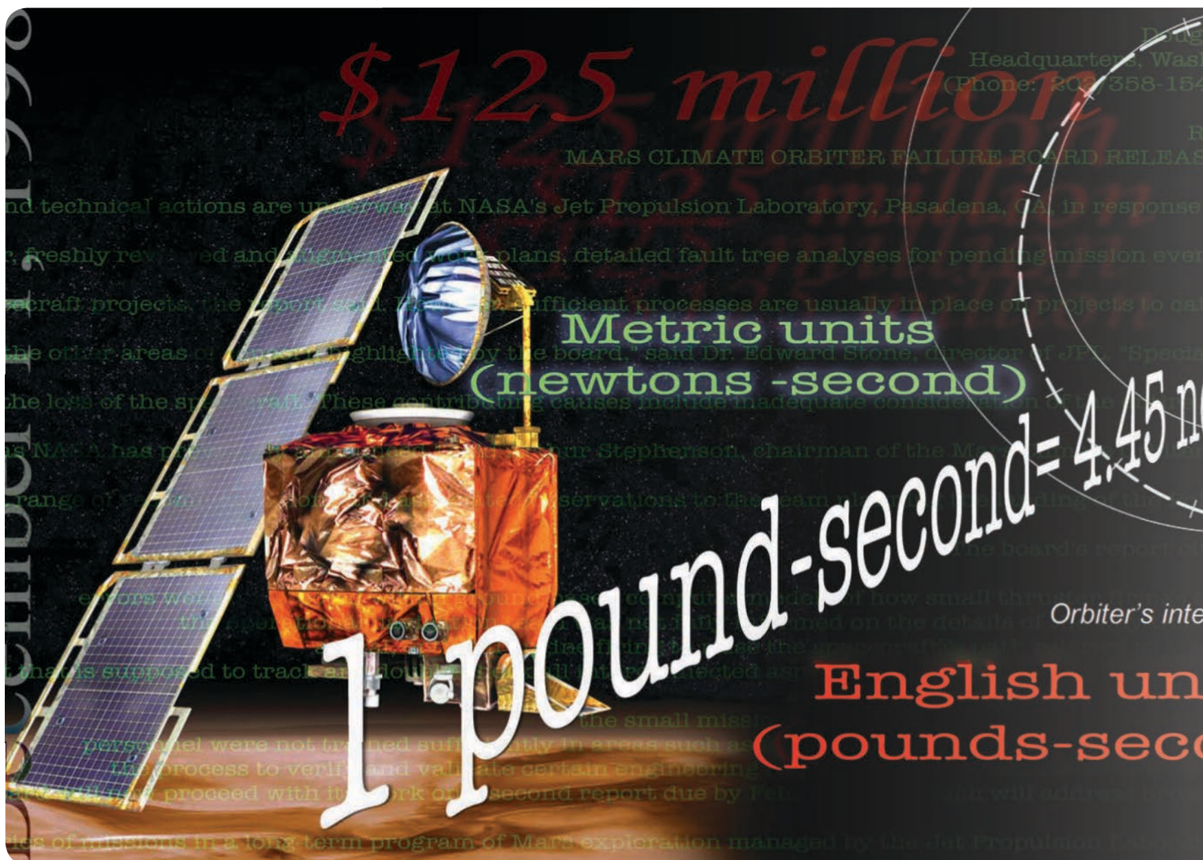
The $125 million Mars Climate Orbiter was lost in the Martian atmosphere in 1999 because of a unit mix-up.
